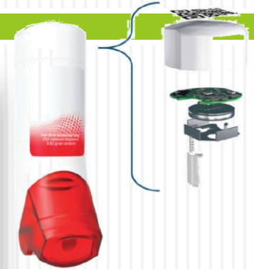
FIG. 1. Exploded schematic view of the Digihaler.
